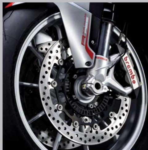
Lightweight design: the wheels of the Brutale 1090 RR are made from aluminium alloy. Designed with thin, slender and elegant spokes, these wheels are manufactured using the best production techniques, in order to ensure the most effective ratio in terms of mechanical properties and weight. And it is precisely their weight that is so impressive, because it has been remarkably reduced exactly where needed. The result? Superior handling for maximum riding pleasure.
